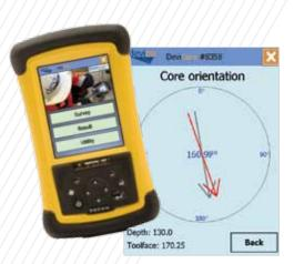
The rock core is orientated at the surface when the two arrows are aligned.
